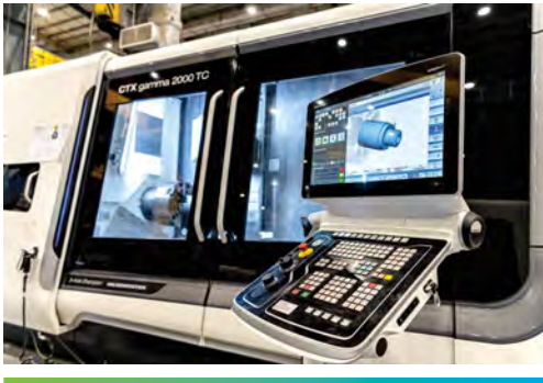
Top: The new MSSD shop in Ju’aymah includes advanced tools, such as this five-axis milling machine, which makes use of computer numerical control technologies to manufacture replacement parts in only hours. Left: Technicians Chris D. Nablo (left) and Sajjad A. Alzayer from the Mechanical Services Shops Department in Ju’aymah are machining the bearing seal in preparation for alignment and repair of a load gear box, using a new Computer Numerical Control Horizontal Boring machine.
