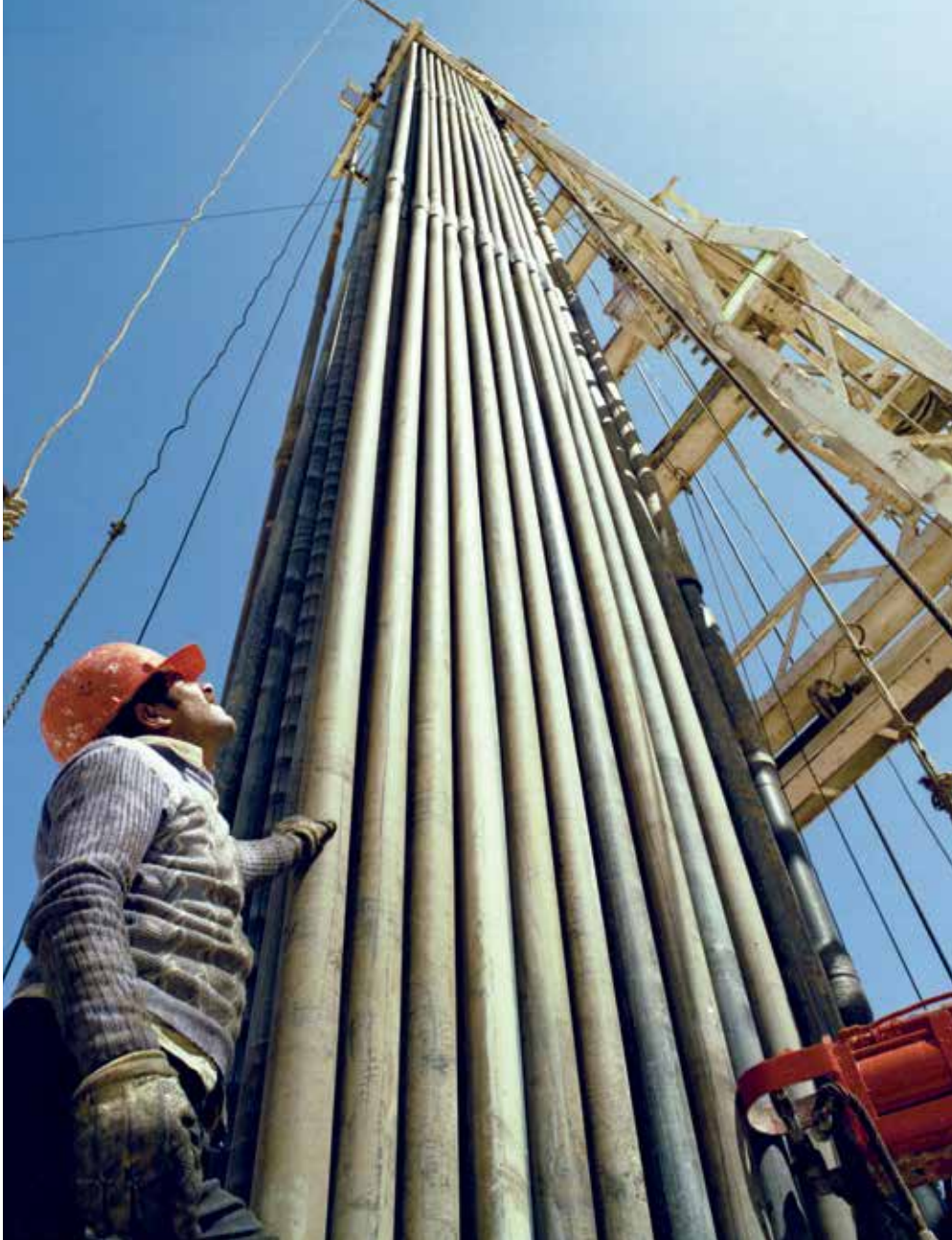
Strings of drill pipe stand ready on a drilling rig at Tamayshah in the Rub' al-Khali in March 1979. This was a test well in the Khuff zone at 3,471 meters and part of Aramco's accelerated gas exploration program in the 1970s.
