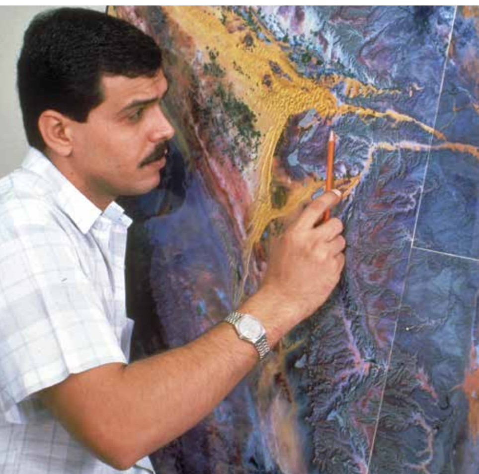
Aramco geologists at EXPEC began utilizing computer-enhanced satellite images, such as this one, recorded by Landsat satellite, 700 kilometers above the Earth. Studying these images allow geologists to identify structural anomalies on the surface that might point to the hydrocarbon traps under the ground.
