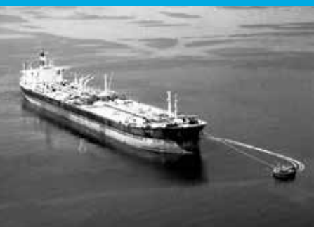
With the Zuluf offshore field entering production in 1973, the F. A. Davies , a converted oil tanker, served as a floating storage vessel.
