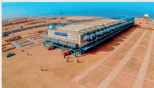
Setting a record that stood for two years, Almajdouie of Dammam, Saudi Arabia, moved the Heaviest Object Transported by Road—a single-piece, 4.9-million kilogram (10.8 million lb) evaporator for a desalination plant.
